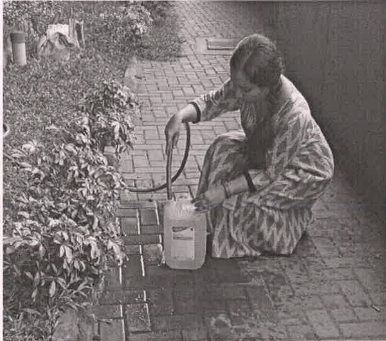
Figure 2.2 Discharge measurement of garden house at station
